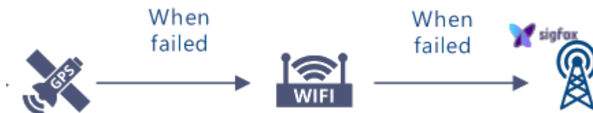
Figure 13 – The procedure for selecting geolocation data for cases of unavailability of certain data
